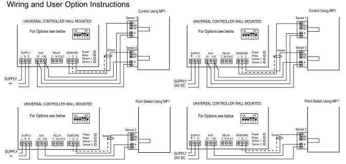
When using MP7 which has a potted 3 core cable, cable colours are as follows Blue = Aux +V, Brown = Aux 0V, Green/Yellow = Sensor
