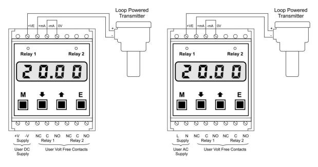
Multi Type 900's can be used for more demanding applications that require additional relay outputs by connecting the transmitter loop in series as follows.
