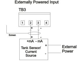
**Note:** If a screened cable is used the screen is typically connected to the Earth terminal at the FXL3NL end only, this is usually for EMI purposes in a noisy environment. If the application requires
