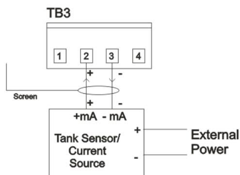
**Note:** If a screened cable is used the screen is typically connected to the Earth terminal at the FXL3NL end only, this is usually for EMI purposes in a noisy environment. If the application requires
