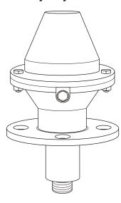
HPE8/P similar to HPE8 but with an insert moulded in, to provide pressure under the flange of 30 psi. Supplied with two rubber gaskets, Stainless Steel nuts and bolts to secure the cap to the base also a Stainless Steel coupler to accept 3/4" pipe electrode.
