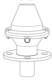
HPE8 Electrode Holder suitable for sewage, water and effluent applications. Moulded in Phenolic (SR4007) for high strength and chemical resistance. Supplied with Stainless Steel clamping collar, rubber gasket and Stainless Steel nuts and bolts to secure the cap to the base. The holders will accept <sup>3</sup>/<sub>4</sub>" pipe electrodes of nominal OD 26.7mm and wall thickness 2.87mm.
