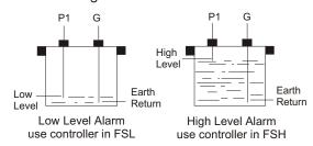
(e.g. pumping out or low level alarm). For control, two active electrodes are used.
