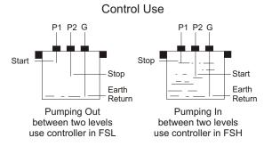
In fail safe high mode (FSH) the controller relay de-energises when the liquid touches the shortest electrode (e.g. pumping in or high level alarm).
